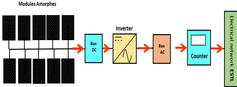
Figure 3 : Block diagram of the entire photovoltaic system
